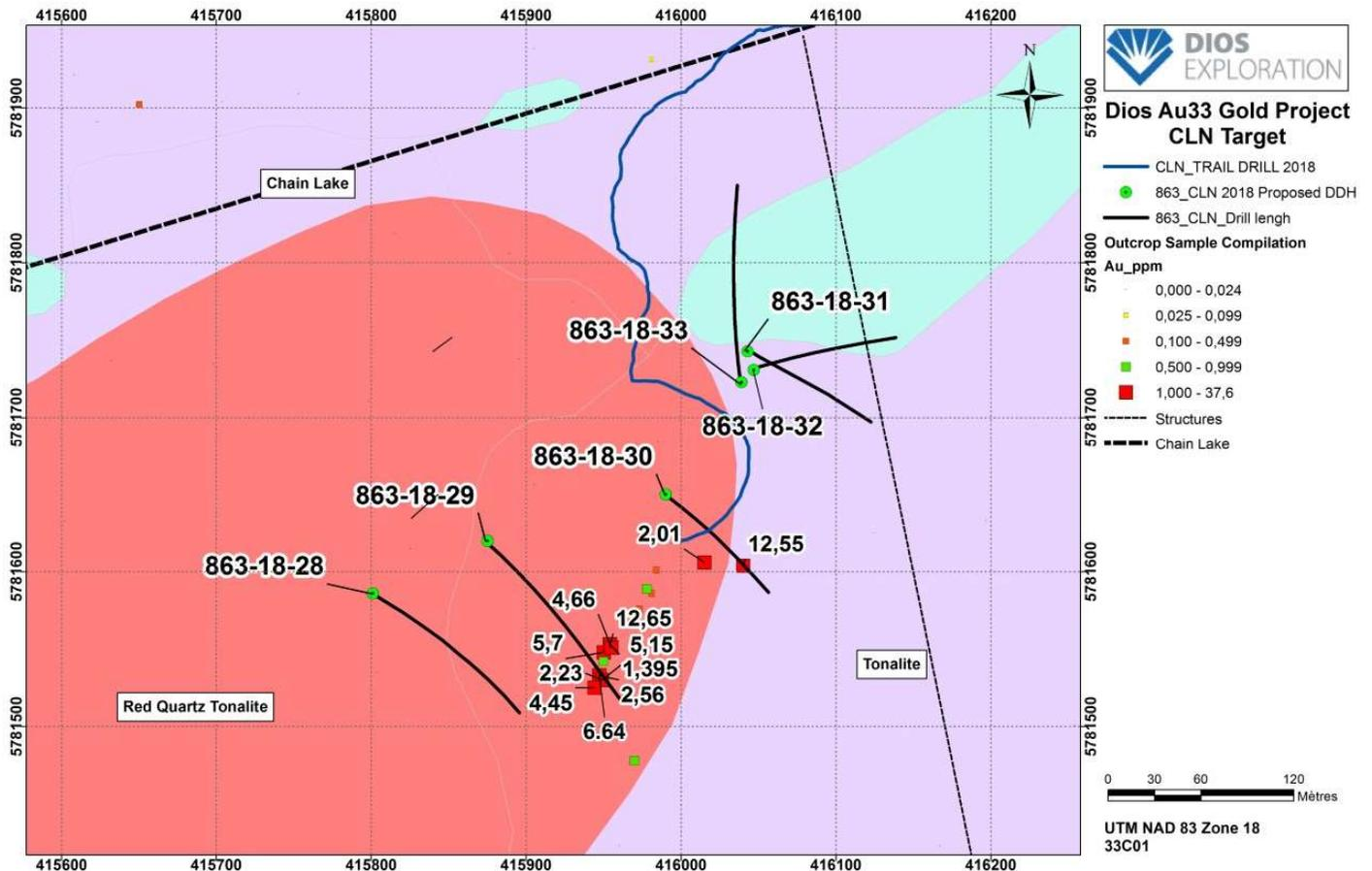
Some 2,326 metres of NQ diameter diamond drilling was completed for gold in 2018: eleven holes completed with success and two lost in the Chain Lake Break.
