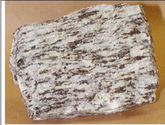
Fig.5: Alaskite gneiss in the central zone of Damara, Namibia, Host-rock of Rossing deposit (from the web-site)
